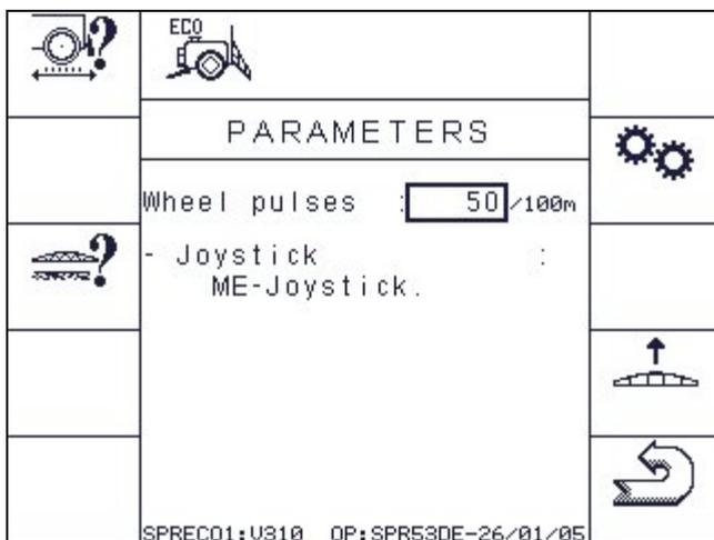
In the parameter mask it is possible to set the wheel pulses per 100 m and it can be selected if a multifunction grip (MFG) is available. The available soft keys call up different calibration masks. See the description in Tab. 4-2.
