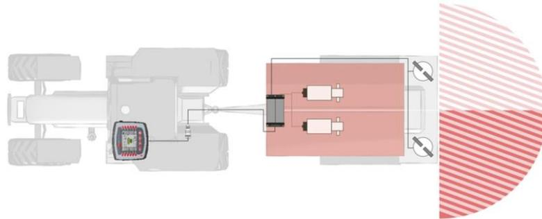
*Example of a fertilizer spreader: The same fertilizer is spread on the left and right. The rate depends on the prescription map.*
