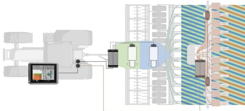
Example of a slurry tanker and planter/seeder: Processing based on different prescription maps.
