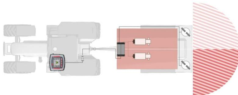
*Fertilizer spreader: The same fertilizer is spread on the left and right. The rate depends on the prescription map.*
