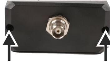
2. Slide the lid of the junction box carefully to the back.
