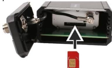
5. If you want to remove the SIM card again, press it inwards a little bit. The SIM card will then be ejected.
