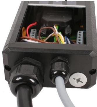
3. Replace the blanking plug from the power supply connector with a grommet.
