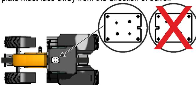
4. Place the GPS receiver onto the magnetic plate so that it locks. The connection must thus face away from the direction of travel.
