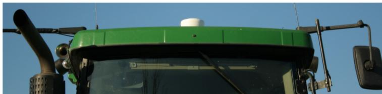
*GPS receiver on the roof of a tractor*
