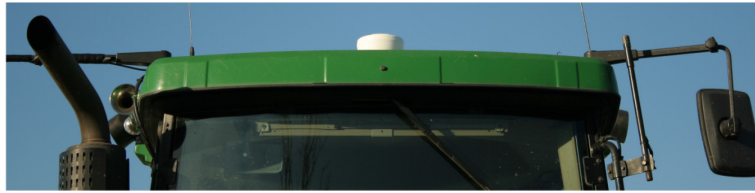
GPS receiver on the roof of a tractor
