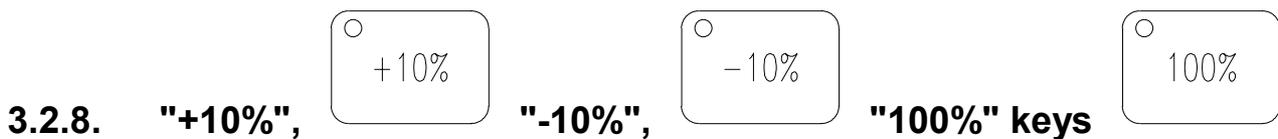
With the "+10%" and "-10%" keys it is possible during operation to vary the spray rate (e.g. liquid manure) in degrees of 10% in relation to the pre-set rate.
