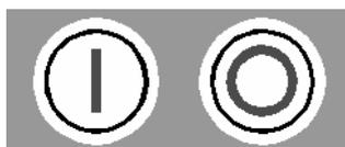
The Unit is switched on with the (I)-key.
