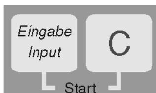
You start the system by pressing the keys "Enter" and "C" simultaneously. To the system this means, that the memory for the area, the time and the distance will be cleared.
