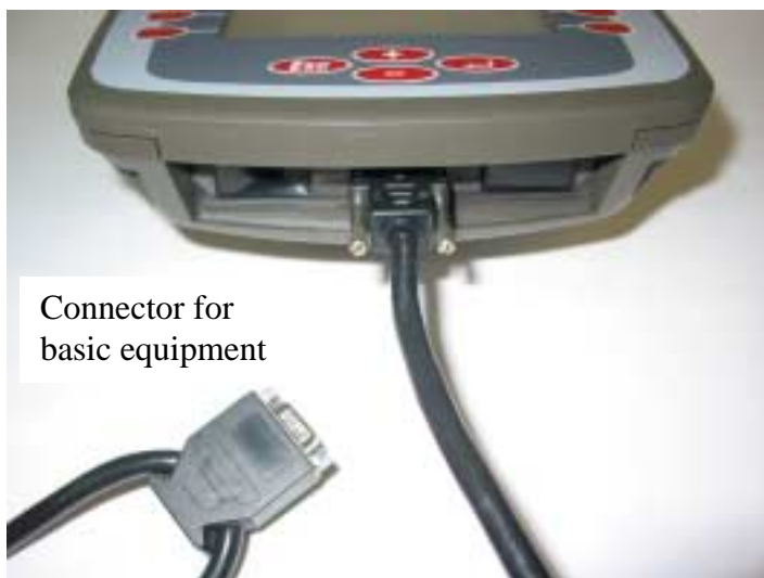
Diagr. 3-8 ECO - Terminal with MFG connecting cable and connection for the basic equipment
